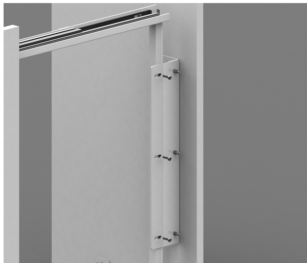
Step 04 Fix the door bracket with frame using fitting kit-2.
