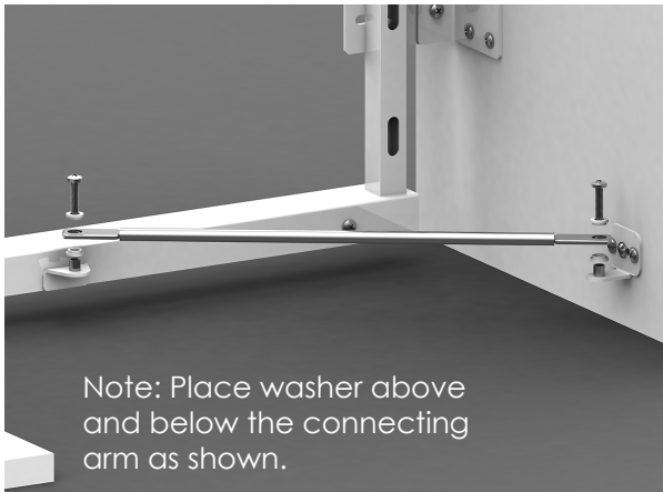
Step 06 With the help of connecting arm connect frame and door connecting arm holder using fitting kit-3.
