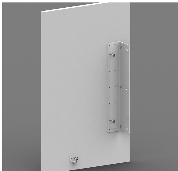
Step 03 Fix the door bracket and door connecting arm holder with door with only 3 screw for further adjustment using door drawing and fitting kit-2.
