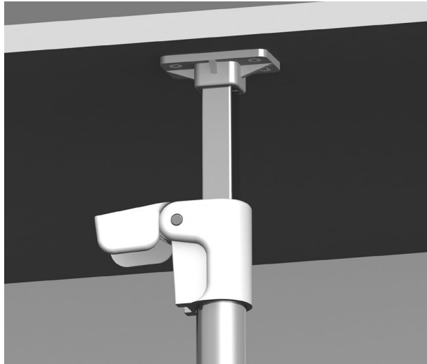
Step 12 : Pull the Square Pipe upto the Pipe Top Bracket as shown in picture.
