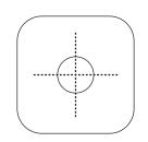
Marking point for fixing screw.
